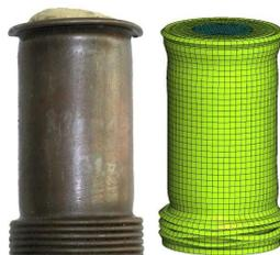
Fig 3. The comparison of numerical and real specimen deformation mode
