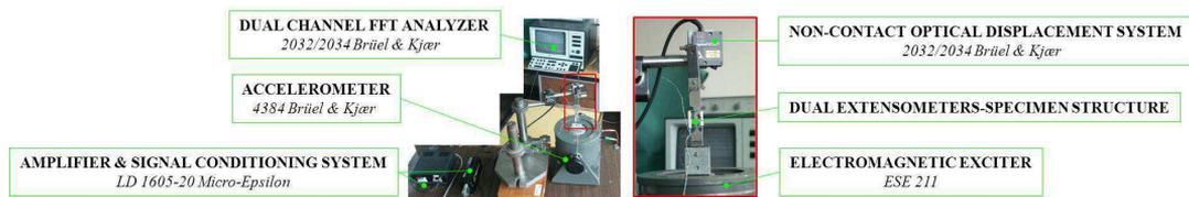
Figure 4. Special measurement path to verify of extensometer-specimen structure natural frequency
