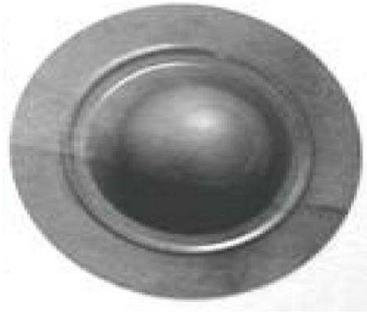
Fig. 2: The experimentally deformed shape of sheet metal
