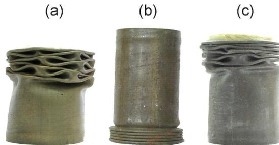
Fig 2. Specimen deformation modes.
